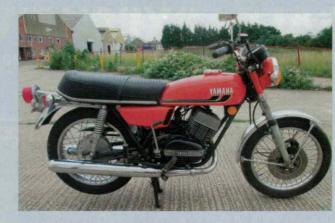
steel frame and a doublepiston front disc brake completed the competent package.
